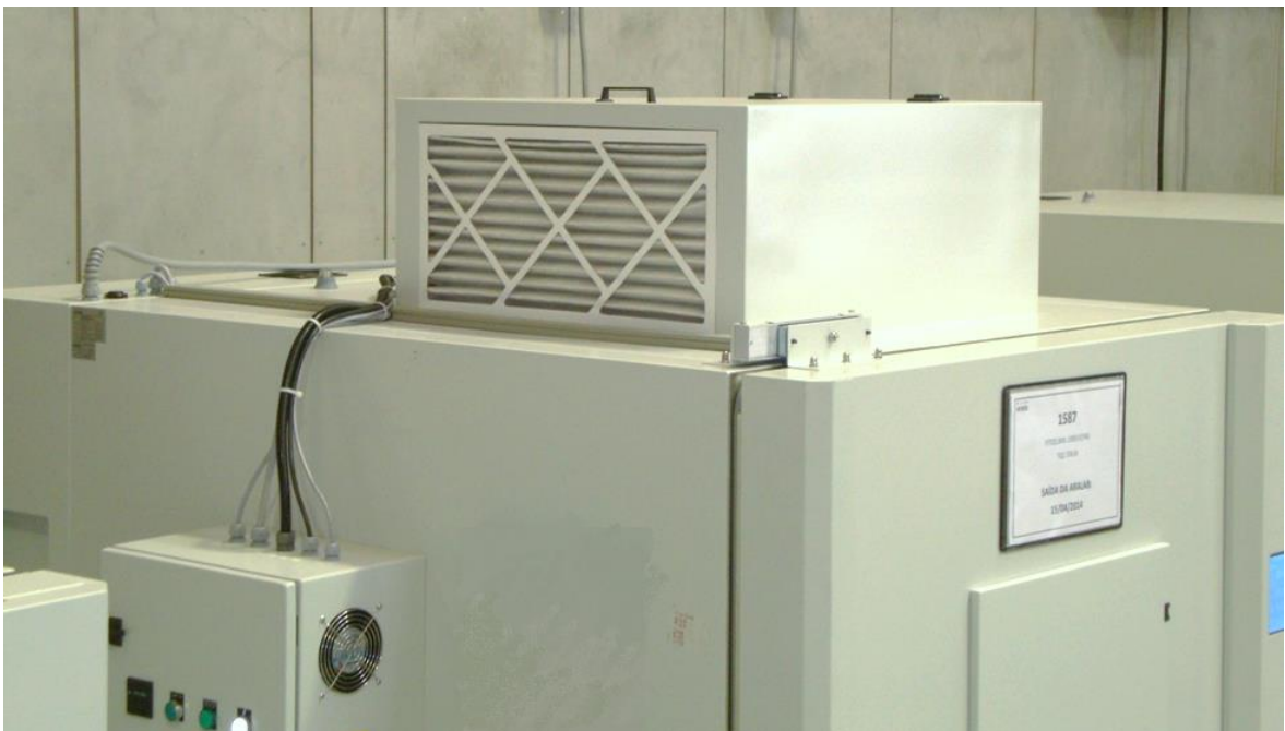
External view of chamber ceiling with lamp accessory and control board (left side). Door with cover lid.
