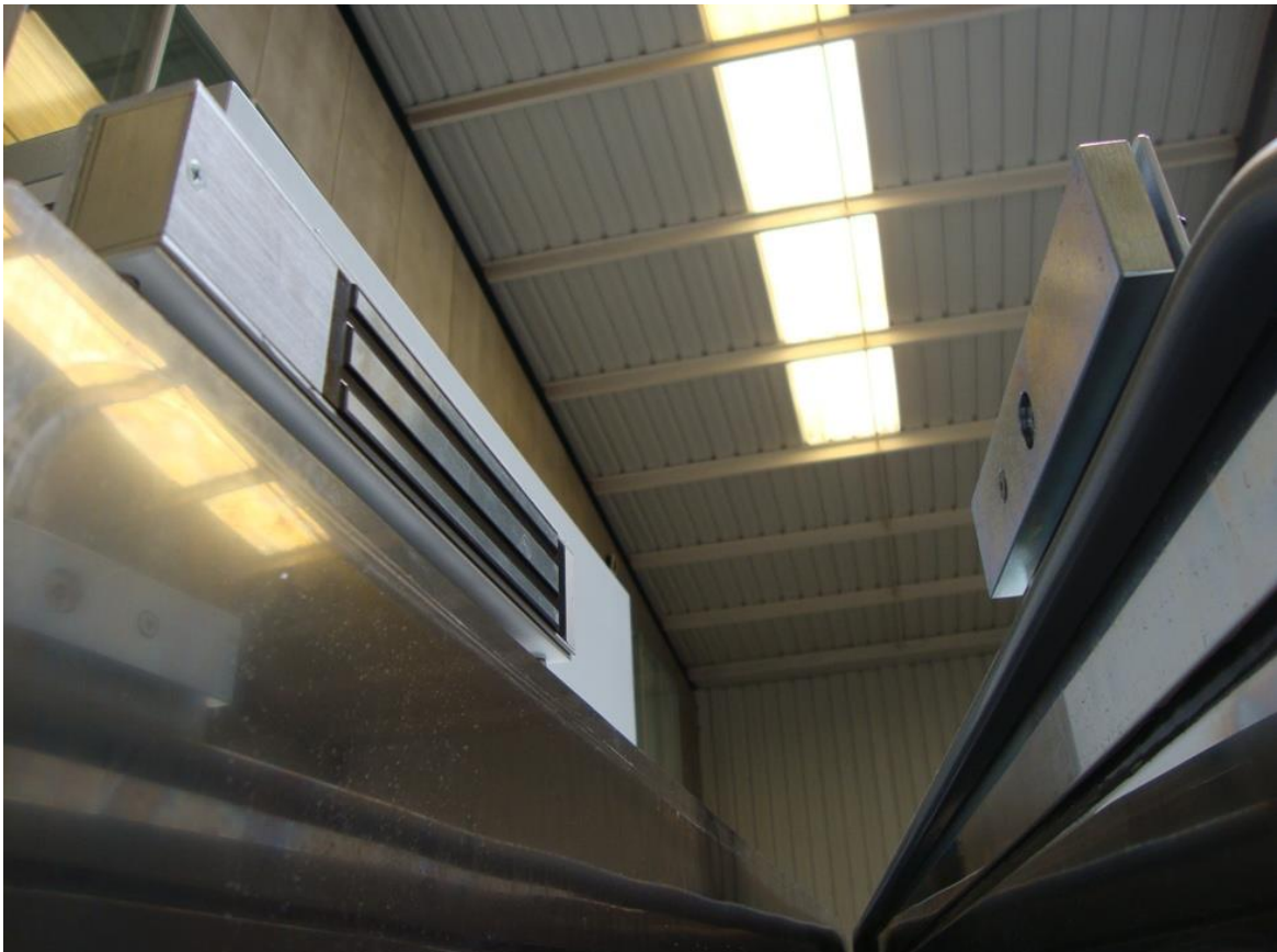
Magnetic door lock integrated with control board securing the chamber door is not opened during test cycles
