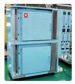
Usage: in battery manufacturing engineering, vacuum drying to remove the moisture and solvent in the electrode material.
