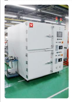
Usage: in battery manufacturing engineering, vacuum drying to remove the moisture and solvent in the electrode material.
