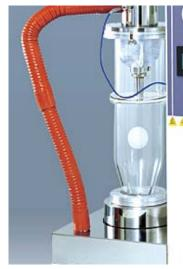
Employment of one touch removal system has made removal or cleaning of the drying chamber, the cyclone, or the product container further easier.
