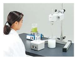
■ Granulation, drying, mixing of powder
