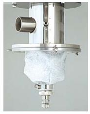
The tip of the nozzle comprises of a nozzle for liquid and a nozzle for gas.
