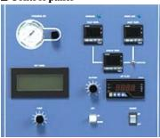
Inlet temperature, outlet temperature, and drying air amount are digitally displayed. Setting is made on the touch panel that allows operation settings, operation status display as well as error display, and settings of various operation conditions also in English and Chinese in addition to Japanese.
