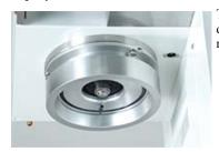
The tip of the nozzle comprises of a nozzle for liquid and a nozzle for gas.
